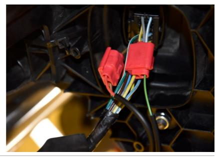
Connect the GPX Black/Green wire to the Red wire of the crankshaft position sensor connector.
