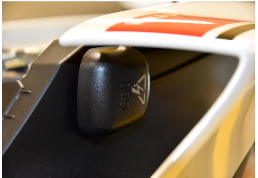
Typical position for the iLE module.
