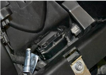
Plug the MM connector to the OBD connector.
