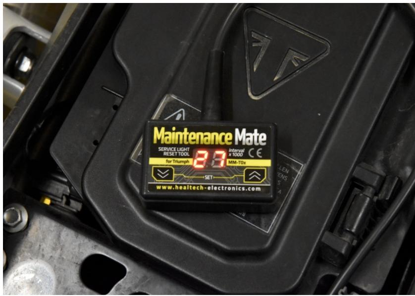
The service lamp disappears and the new service interval is loaded.
