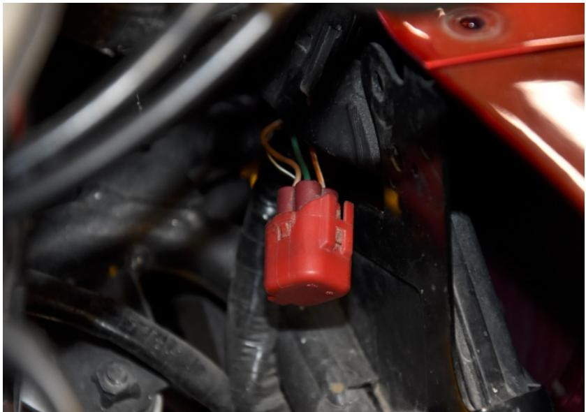
Plug the OBD connector to the the diagnostic system connector and the USB connector to the computer.
