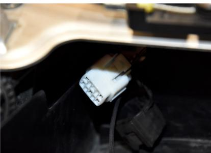
Plug the OBD connector to the the diagnostic connector and the USB connector to the computer.
