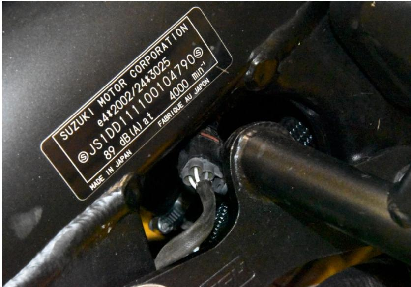
Plug the OSE connector into the wiring harness connector.
