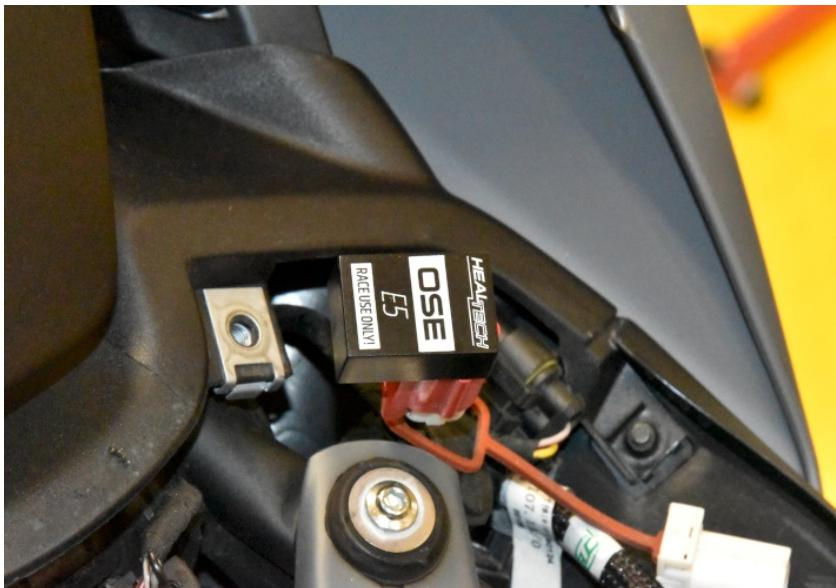
Secure the red connector properly with a cable tie.
