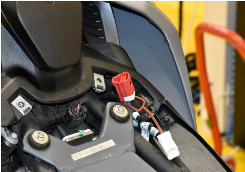
Plug the OSE-E5 module to the diagnostic connector.
