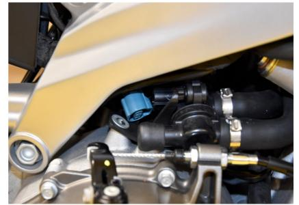
Plug the PSE module into the wiring harness connector.
