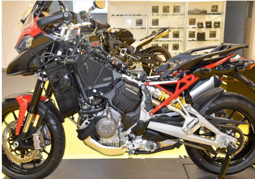
Locate the stock PAIR (clean air) valve under the fuel tank.
