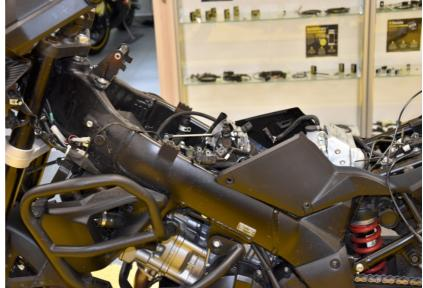
Locate the stock PAIR (clean air) valve under the airbox on the right side and unplug the connector.
