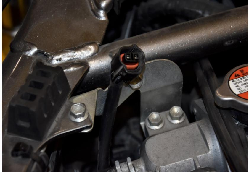
Plug the PSE module into the wiring harness connector.
