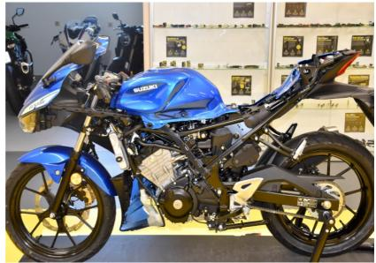
Locate the stock PAIR (clean air) valve under the fuel tank and unplug the connector.
