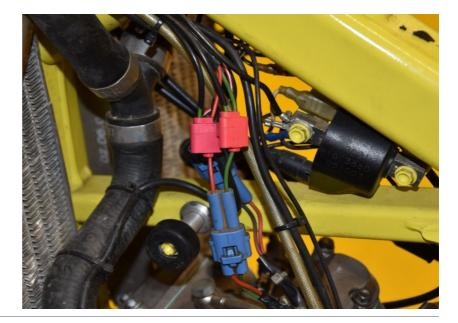
Connect the QSH Black wire terminal to the ignition coil ground terminal.
