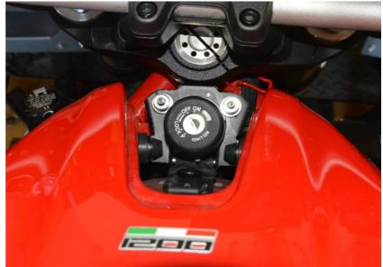
Lift up or remove the fuel tank.
