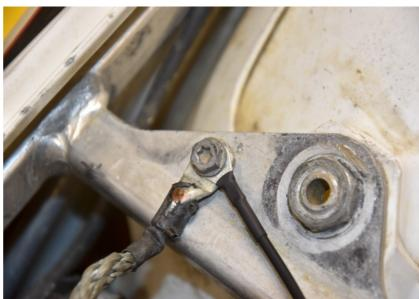
Mount the QSE sensor under the bolt of gearbox shaft.
