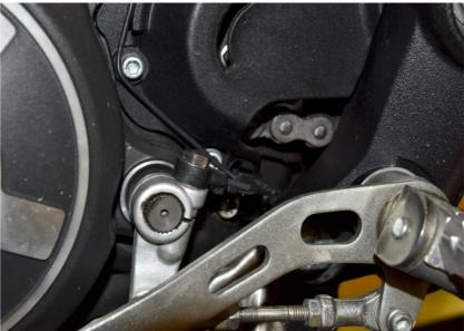
Typical position for the QuickShifter easy. Secure the unit Properly.
