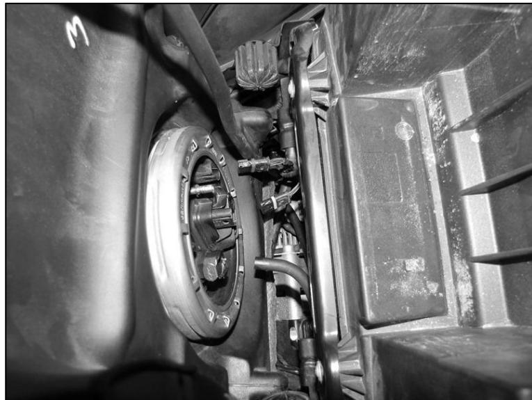
2.4.- Remove the overfill rubber hose from the top of the tank and then remove the tank completely.
