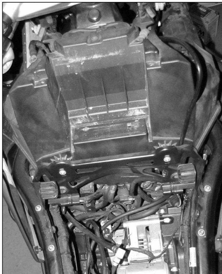
**3.- Remove Intake runner with filter**, by unclipping the two plastic clips.
