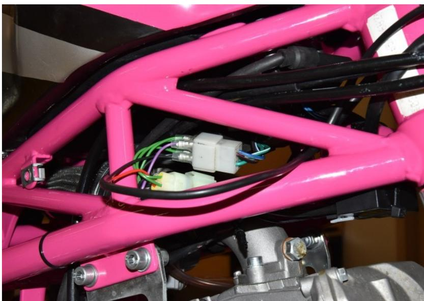
Use the supplied black jumper cable to make a ground connection between the engine and the ignition coil's ground terminal.
