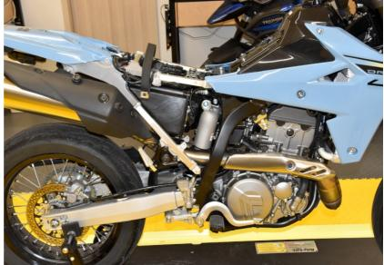
Locate the ignition coil connectors under the the fuel tank.
