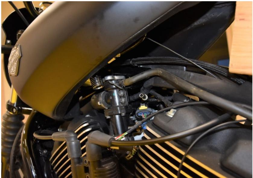
Locate the ignition coil connector
