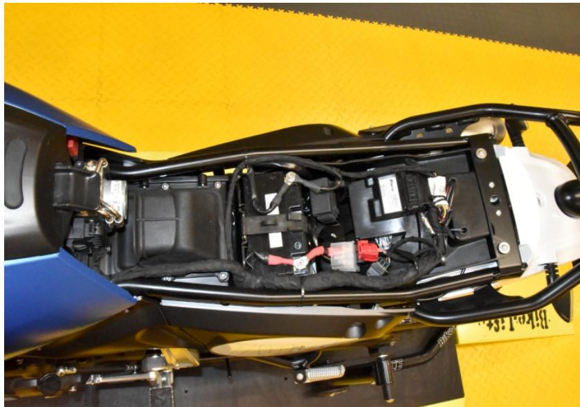
Plug the QSH connectors in-line with the ignition coil connectors.
