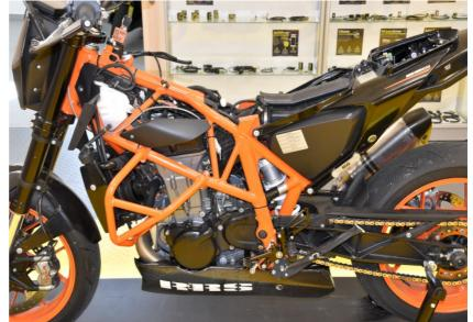
Locate the ignition coil connectors on the right side.
