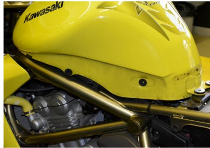
Lift up or remove the fuel tank.
