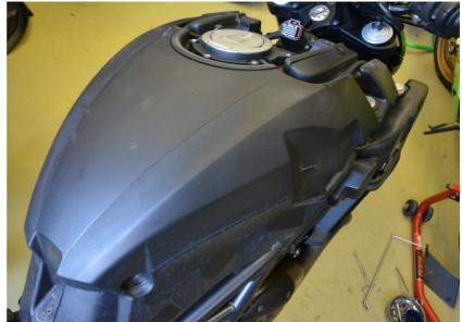
Remove or lift up the fuel tank.
