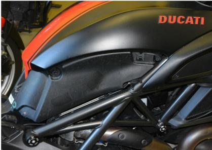
Remove the airbox intake covers from the left and right side.
