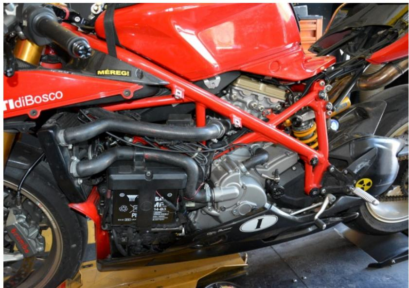
Plug the QSH connectors in-line with the ignition coil connectors of the front cylinder.
