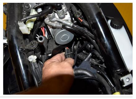
Connect the QSH connectors in-line with the ignition coil connectors.
