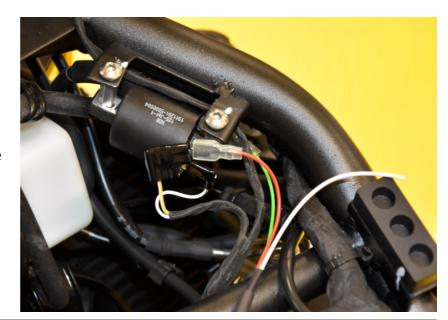
Splice the QSH White wire to the White/Black wire of the coil by using the supplied red wire tap connector.
