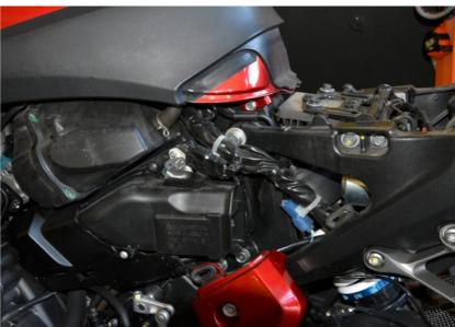
Lift up or remove the fuel tank.
