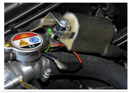
Splice the QSH White wire to the Yellow/Blue wire of the coil by using the supplied red wire tap connector.
