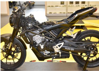
Locate the ignition coil connectors under the fuel tank.
