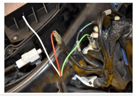
Splice the QSH White wire to the Green/Blue wire of the coil by using the supplied red wire tap connector.
