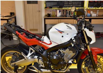
Locate the ignition coil connectors on the right side under the side fairing.
