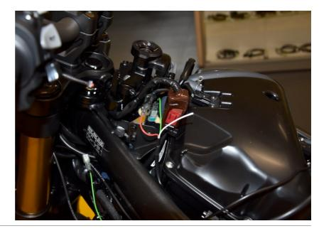
Splice the QSH White wire to the Green/White wire of the coil by using the supplied red wire tap connector.
