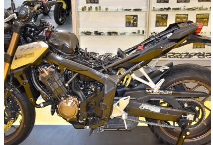
Locate the ignition coil connectors under the fuel tank.
