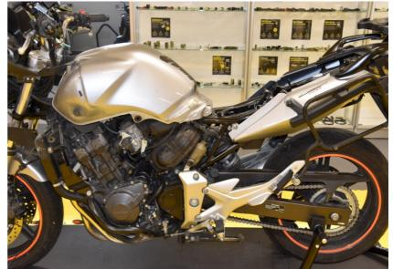
Locate the ignition coil connectors on the right side under the fuel tank.
