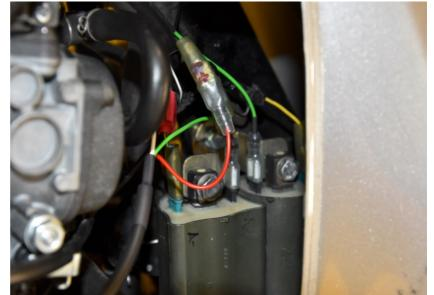
Connect the QSH Black wire terminal to the battery negative terminal.
