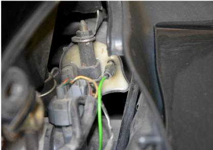
Splice the QSH White wire to the Yellow/Blue or Blue/Yellow wire of the coil by using the supplied red wire tap connector.
