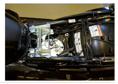
Lift up or remove the fuel tank.
