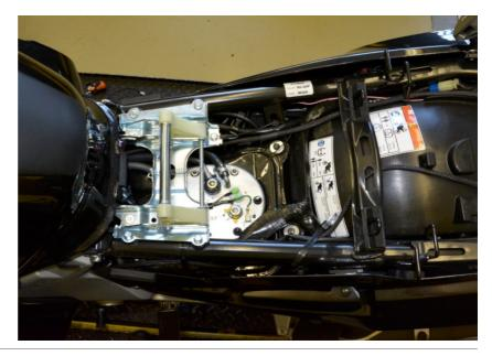
Lift up or remove the fuel tank.
