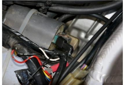
Splice the QSH White wire to the Black/White wire of the Crankshaft Position Sensor connector by using the supplied red wire tap connector.
