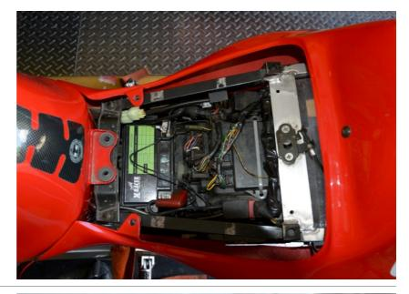
Lift up or remove the fuel tank.
