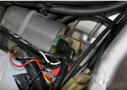
Splice the QSH White wire to the Black/White wire of the Crankshaft Position Sensor connector by using the supplied red wire tap connector.
