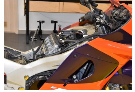
Locate the ignition coil terminals under the fuel tank on both sides.
