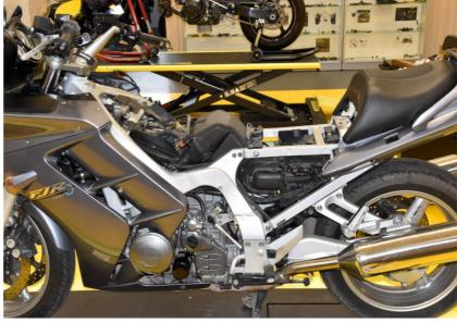
Locate the ignition coil connectors under the side panel on the right side.
