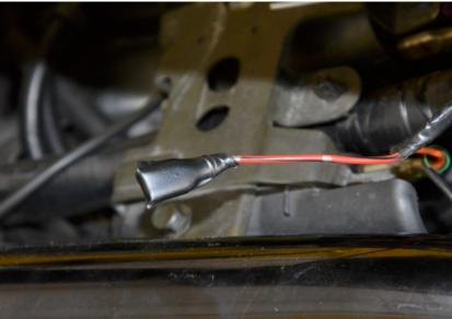
Splice the QSH White wire to the Gray wire of the coil by using the supplied red wire tap connector.
