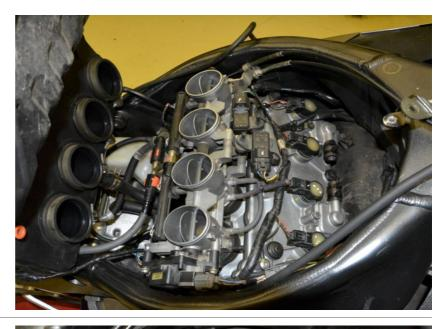
Plug the QSH connectors in-line with the ignition coil connectors.
