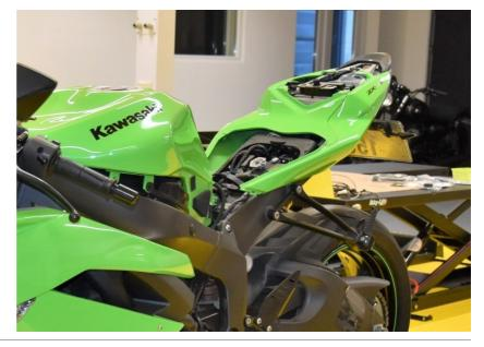
Remove or lift up the fuel tank.
