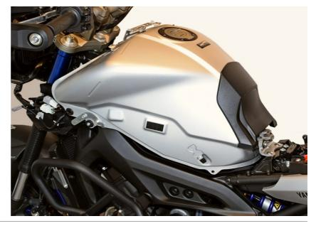
Remove the fuel tank and the airbox.
