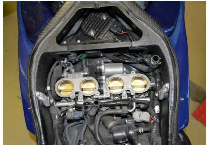
Remove the voltage regulator with the plastic holder.
