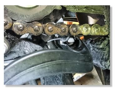
REPLACE THE BOLT WITH THE ONE SUPPLIED.
