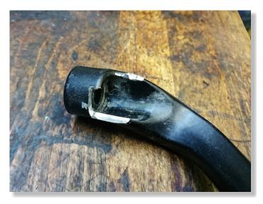
THIS MOTORCYCLE HAS A UNIQUE SHIFT ARM WHICH IS NOT COMPATIBLE WITH ANY QUICK SHIFTER SENSORS ON THE MARKET WITHOUT MODIFICATIONS. TO INSTALL THE QSE SENSOR, TAKE OFF THE SHIFT ARM FIRST AND USE AN ANGLE GRINDER TO MAKE ROOM FOR THE SENSOR. MAKE SURE THE NECK OF THE SENSOR DOES NOT TOUCH THE METAL LEVER AT ANY POINT.
