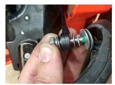
TIGHTEN THE BOLT IN THIS POSITION BY ABOUT 6 NM.
