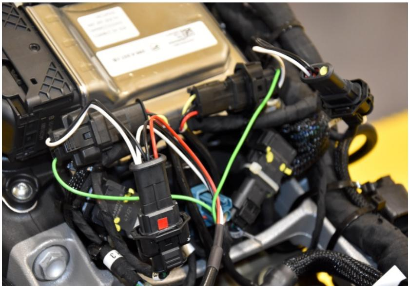
Plug the QSH connectors in-line with the ignition coil connectors on the vertical cylinders.
