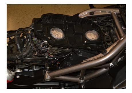
Connect the QSH connectors in-line with the ignition coil connectors on the left side.
