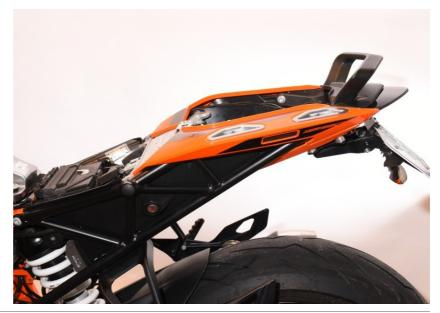
Remove the left and right side covers with the blinkers.
