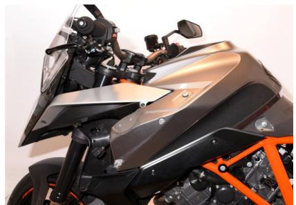
Remove the lower plastic covers around the fuel tank.
