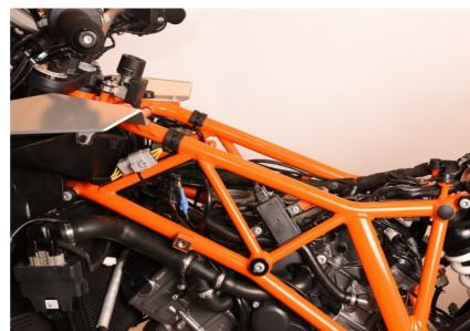
Connect the QSH connectors in-line with the fuel injector connectors.
