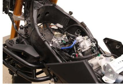
Plug the QSX connectors in-line with the fuel injector connectors.
