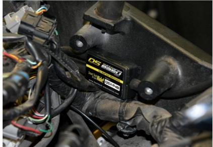
Connect the QSX Black wire terminal to the battery negative terminal.
